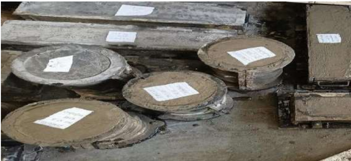
Fig 6 Casting of concrete cylinders & prism using paper sludge as a self-curing agent
