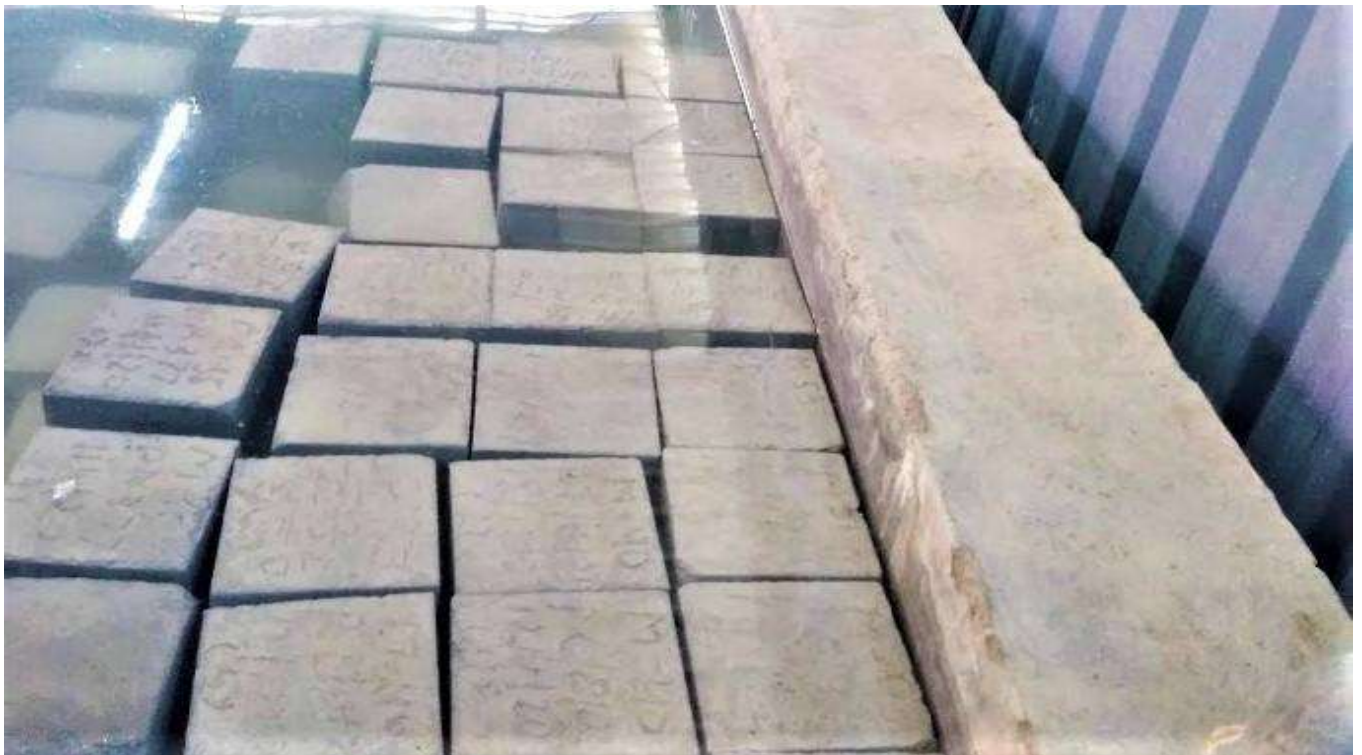
Fig 9 Curing of concrete cubes for normal concrete
