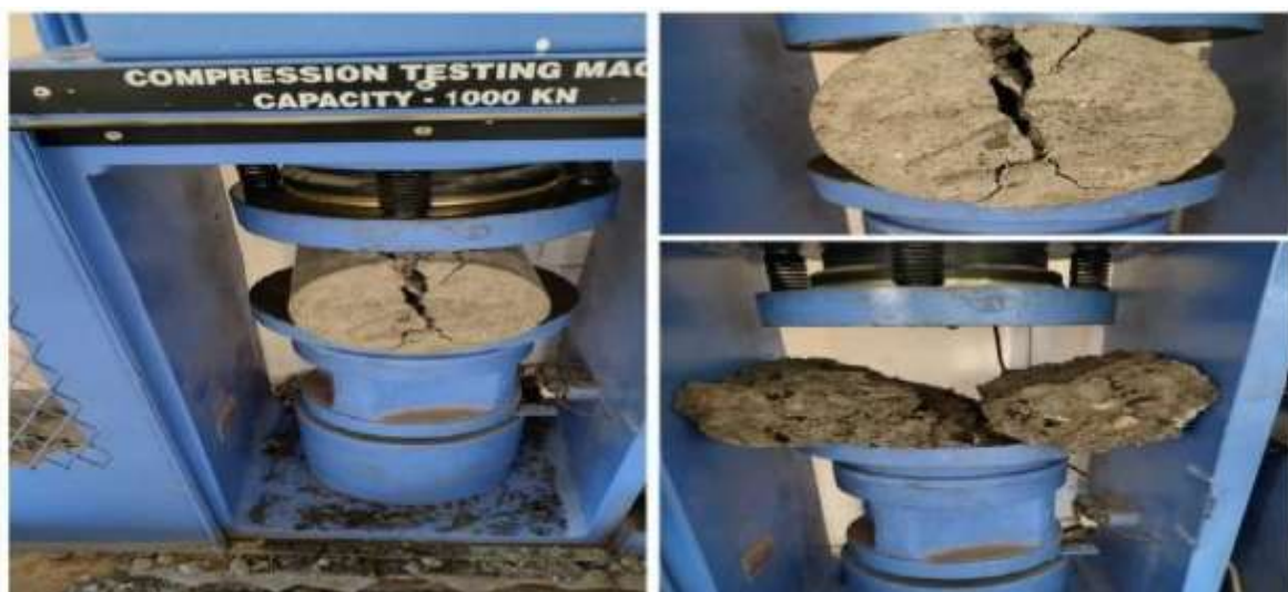
Fig 7 Split Tensile testing of concrete by using paper sludge as a self-curing agent
