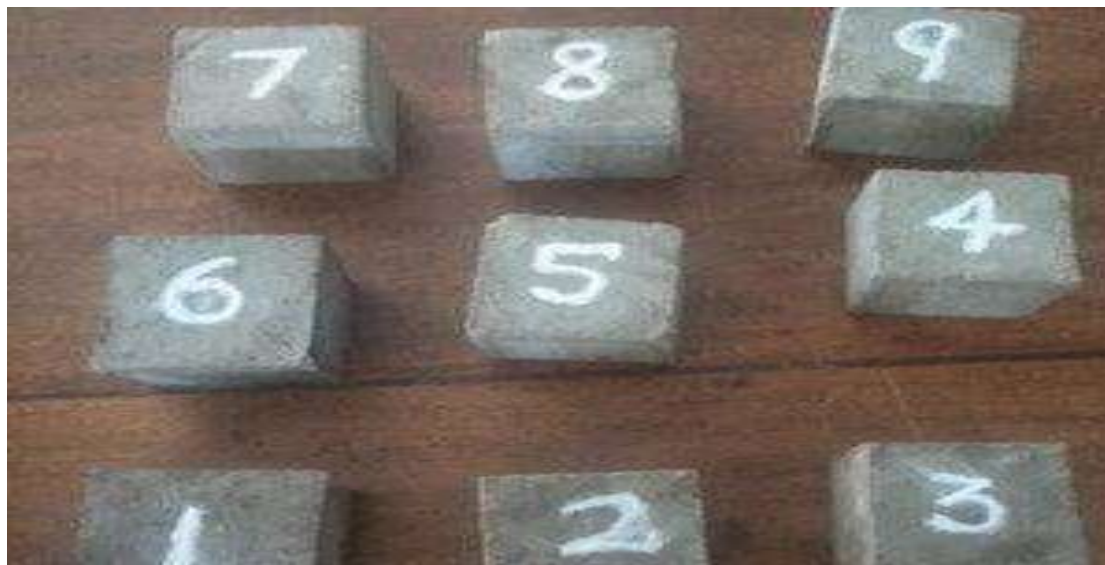
Fig 4 Casting of concrete cubes by using paper sludge as a self-curing agent
